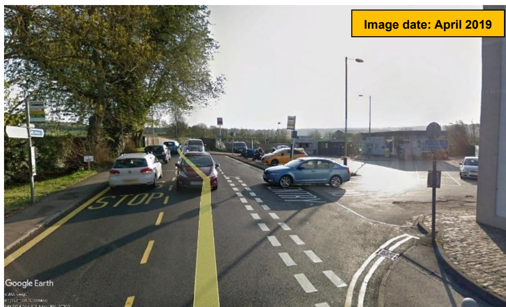
Figure 5-16: Lack of pedestrian crossing across Station Road outside Tring railway station
