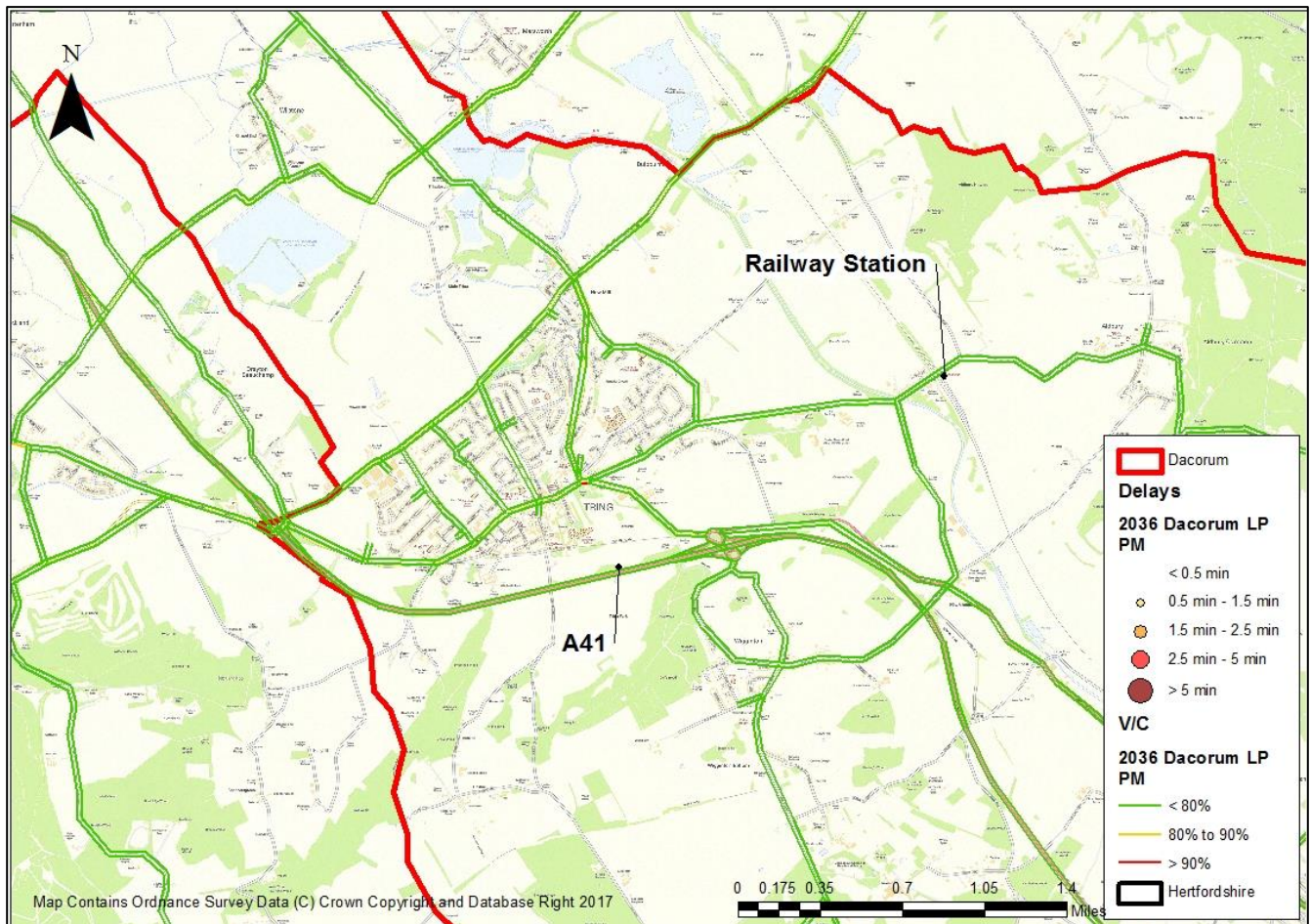
Figure 31: Delays and Link Stress around Tring in the 2036 Dacorum Local Plan Scenario – PM peak
