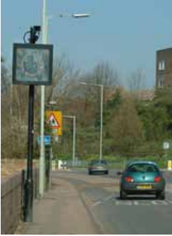
A Vehicle Activated (VA) sign to warn drivers about their speed
