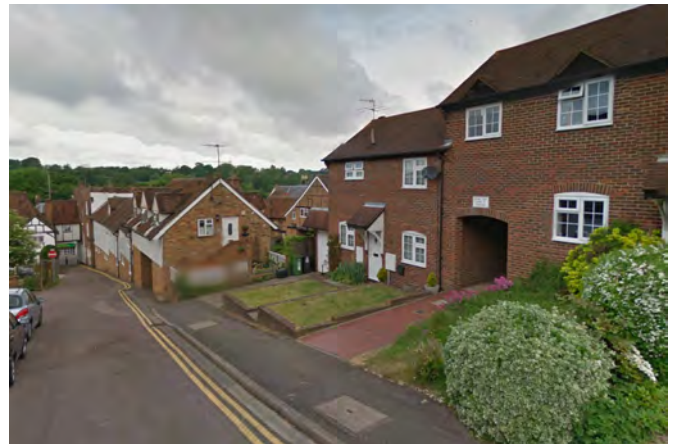
Figure 33: The existing homes on the nearby Chapel Street step down the steep hill and provide level access for each dwelling. Front gardens are terraced with the levels of the road
