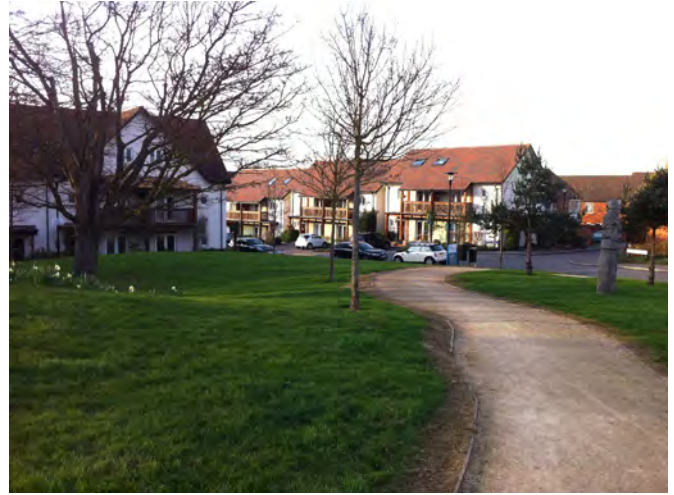
Figure 32: The buildings in this example step down with the topography of the site and the open space has been designed to incorporate existing levels and features
