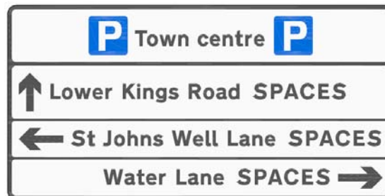
Figure 9 Example High Street West VMS Sign
